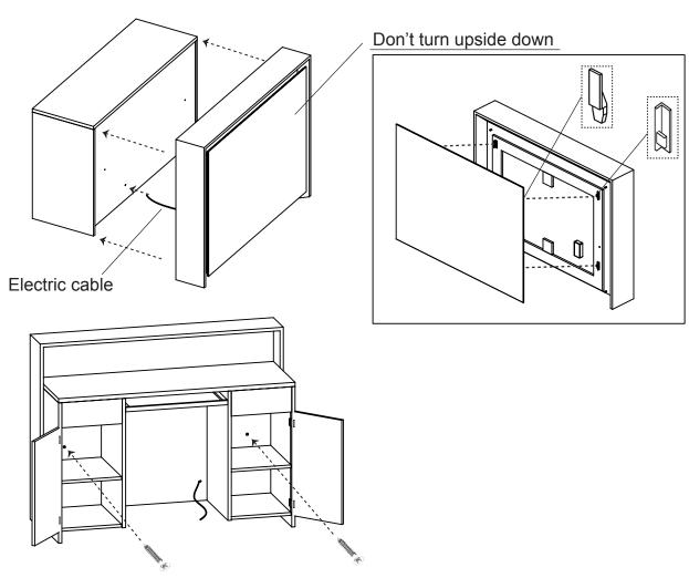
3 Wire the LED switch to Electric cable.
